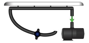
Locate the Reservoir Lid. On the under side of the lid, locate the open end of the black tubing. Attach the end of the tubing to the connector on the top of the Water Pump. Retun the lid to the Reservoir.
